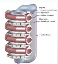
Figure 1. Thermoacoustic piezeelectric generator, consisting of four thermoacoustic Stirling engines driving four piezeelectric alternators
