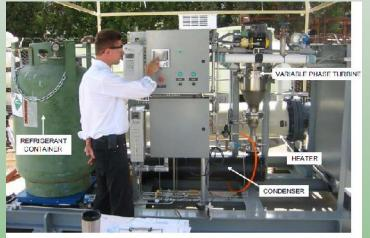
Figure 12. Variable Phase Turbine operating in pilot plant.
